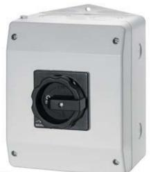
MAIN CONTROL SWITCH 3-POLE IU=63, P/AC-23A AT 400V=22KW 1 N-TERMINAL + 1 PE-TERMINAL ENCAPSUL.IN M.P.ENCLOSURE, IP65 ROTARY ACTUATOR BLACK METRIC THREAD
