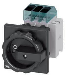
Switch disconnector 3LD3, main switch 3-polig, lu 16A operational switch at AC-23 A at 400 V 7,5 kW front mounted Base mounting with center-hole 22,5 mm rotary operationg mechanism black 66 x66 mm with auxiliary 1NO+1NC
