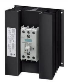
SEMI-CONDUCTOR CONTAC.3-PH.3RF2 AC51 50A 40 DEG. C 48-600V / 4-30V DC 3-PHASE CONTROLLED SCREW TERMINAL BLOCKING VOLTAGE 1200V
