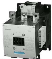
CONTACTOR, 110KW/400V/AC-3 AC(40...60HZ)/DC OPERATION UC 21-27.3V AUXILIARY CONTACTS 2NO+2NC 3-POLE, SIZE S10 BAR CONNECTIONS ELECTRONIC OPERATING MECHANISM WITH 24 V DC PLC INTERFACE CAGE CLAMP TERMINAL
