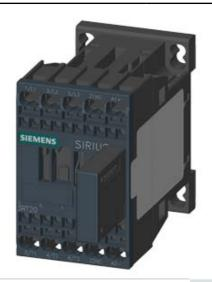
COUPLING RELAY, AC-3, 5.5 KW/400 V, 1NC, DC 24V, 0.85...1.85 \*US, W. PLUGGED-ON VARISTOR 3-POLE SZ S00, SPRING-LOADED TERMINAL
