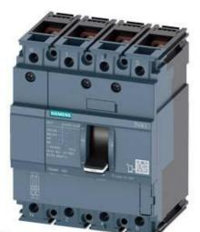
CIRCUIT BREAKER 3VA1 IEC FRAME 160 BREAKING CAPACITY CLASS S ICU=36KA @ 415 V 4-POLE, LINE PROTECTION TM210, FTFM, IN=125A OVERLOAD PROTECTION IR=125A FIXED SHORT CIRCUIT PROTECTION II=10 X IN NEUTRAL PROTECTION 50% BUSBAR CONNECTION
