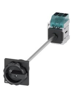
Switch disconnector 3LD3, main switch 3-polig, lu 16A operational switch at AC-23 A at 400 V 7,5 kW floor mounting Base mounting with door coupling center-hole 22,5 mm rotary operationg mechanism black 66 x66 mm with auxiliary 1NO+1NC
