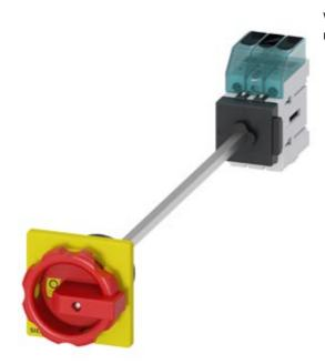
Switch disconnector 3LD3, main switch 3-polig, lu 32A operational switch at AC-23 A at 400 V 11,5 kW floor mounting Base mounting with door coupling center-hole 22,5 mm rotary operationg mechanism red/yellow 66 x66 mm
