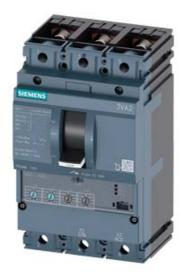
CIRCUIT BREAKER 3VA2 IEC FRAME 100 BREAKING CAPACITY CLASS C ICU=110KA @ 415 V 3POLE, LINE PROTECTION ETU330, LIG, IN=100A OVERLOAD PROTECTION IR=40A ...100A SHORT CIRCUIT PROTECTION II=1,5...12 X IN GROUNDFAULTPROTECTION IG=0,2... 1 X IN, TG=0,1/0,3MS BUSBAR CONNECTION
