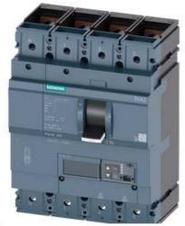
CIRCUIT BREAKER 3VA2 IEC FRAME 400 BREAKING CAPACITY CLASS M ICU=55KA @ 415 V 4-POLE, LINE PROTECTION ETU560, LSIG, IN=400A OVERLOAD PROTECTION IR=160A ...400A SHORT CIRCUIT PROTECTION ISD=0,6..10X IN, II=1,5..10X IN NEUTRAL PROTECTION ADJUSTABLE (OFF, UPTO 100%) GROUND-FAULT, SWITCHABLE IG=0,2... 1 X IN, TG=0,05-0,8MS BUSBAR CONNECTION
