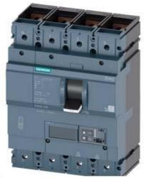
CIRCUIT BREAKER 3VA2 IEC FRAME 630 BREAKING CAPACITY CLASS C ICU=110KA @ 415 V 4-POLE, LINE PROTECTION ETU850, LSI, IN=400A OVERLOAD PROTECTION IR=160A ...400A SHORT CIRCUIT PROTECTION ISD=0,6..10X IN, II=1,5..15X IN NEUTRAL PROTECTION ADJUSTABLE (OFF, UPTO 160%) BUSBAR CONNECTION
