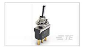
Configuration (Pole-Throw): Single Pole - Double Throw Bushing Thread Size: M6 x .75 Sealed: Yes Contact Base Material: Copper Alloy Switch Contact Plating Material: Gold
