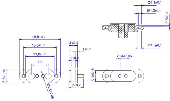
Current Rate : 1A Dimensions : Millimeters
