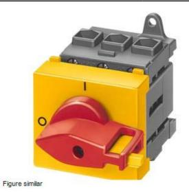
MAIN/EMERG. STOP SWITCH 3-POLE IU=125, P/AC-23A AT 400V=45KW FLOOR MOUNTING DIN RAIL/TWO-HOLE MOUNTING KNOB RED/YELLOW (EMERG. STOP)
