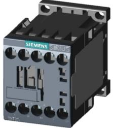
2NO+2NC CONTACTOR, AC3: 7.5KW DC 110V 50HZ, 120V 60HZ 4-POLE, 2NO+2NC, SZ: S00, SCREW TERMINAL
