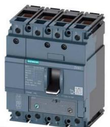
CIRCUIT BREAKER 3VA1 IEC FRAME 160 BREAKING CAPACITY CLASS N ICU=25KA @ 415 V 4-POLE, LINE PROTECTION TM240, ATAM, IN=125A OVERLOAD PROTECTION IR=87,5A ...125A SHORT CIRCUIT PROTECTION II=5...10 X IN NEUTRAL PROTECTION 100% CABLE CONNECTION
