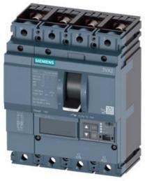
CIRCUIT BREAKER 3VA2 IEC FRAME 160 BREAKING CAPACITY CLASS M ICU=55KA @ 415 V 4POLE, LINE PROTECTION ETU550, LSI, IN=63A OVERLOAD PROTECTION IR=25A ...63A SHORT CIRCUIT PROTECTION ISD=0,6..10X IN, II=1,5..12X IN NEUTRAL PROTECTION ADJUSTABLE (OFF, UPTO 160%) BUSBAR CONNECTION
