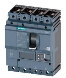
CIRCUIT BREAKER 3VA2 IEC FRAME 160 BREAKING CAPACITY CLASS M ICU=55KA @ 415 V 4POLE, LINE PROTECTION ETU850, LSI, IN=63A OVERLOAD PROTECTION IR=25A ...63A SHORT CIRCUIT PROTECTION ISD=0,6..10X IN, II=1,5..12X IN NEUTRAL PROTECTION ADJUSTABLE (OFF, UPTO 160%) BUSBAR CONNECTION
