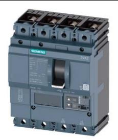
CIRCUIT BREAKER 3VA2 IEC FRAME 250 BREAKING CAPACITY CLASS L ICU=150KA @ 415 V 4POLE, LINE PROTECTION ETU560, LSIG, IN=160A OVERLOAD PROTECTION IR=64A ...160A SHORT CIRCUIT PROTECTION ISD=0,6..10X IN, II=1,5..12X IN NEUTRAL PROTECTION ADJUSTABLE (OFF, UPTO 160%) GROUNDFAULT, SWITCHABLE IG=0,2... 1 X IN, TG=0,050,8MS BUSBAR CONNECTION
