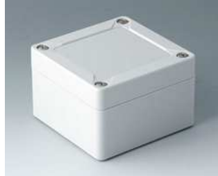
C7008012 IN-BOX PC lichtgrau RAL 7035 84x82x55mm IP 66, IP 67, IK 08
