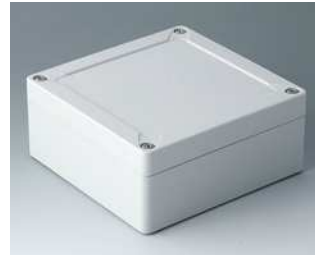
C7013031 IN-BOX ABS (UL 94 HB) lichtgrau RAL 7035 124x122x55mm IP 66, IP 67, IK 07
