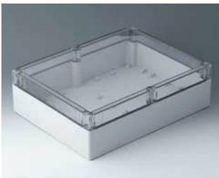
C7030104 IN-BOX ABS/PC (UL 94 HB) lichtgrau RAL 7035 302x232x90mm IP 66, IP 67, IK 07
