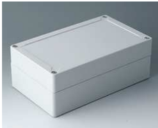
C7020041 IN-BOX ABS (UL 94 HB) lichtgrau RAL 7035 202x122x75mm IP 66, IP 67, IK 07
