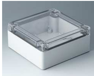
C7013035 IN-BOX PC lichtgrau RAL 7035 124x122x55mm IP 66, IP 67, IK 08
