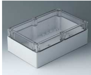
C7025084 IN-BOX ABS/PC (UL 94 HB) lichtgrau RAL 7035 252x162x90mm IP 66, IP 67, IK 07
