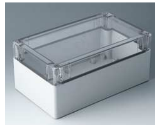
C7020065 IN-BOX PC lichtgrau RAL 7035 202x122x90mm IP 66, IP 67, IK 08
