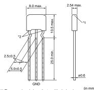
\*1 There may be a hole on the top of ferrite beads, which cause no characteristics deterioration.
