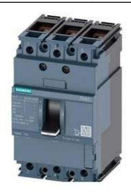
CIRCUIT BREAKER 3VA1 IEC FRAME 160 BREAKING CAPACITY CLASS N ICU=25KA @ 415 V 3-POLE, LINE PROTECTION TM210, FTFM, IN=32A OVERLOAD PROTECTION IR=32A FIXED SHORT CIRCUIT PROTECTION II=10 X IN BUSBAR CONNECTION
