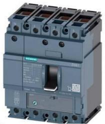
CIRCUIT BREAKER 3VA1 IEC FRAME 160 BREAKING CAPACITY CLASS H ICU=70KA @ 415 V 4-POLE, LINE PROTECTION TM220, ATFM, IN=40A OVERLOAD PROTECTION IR=28A ...40A SHORT CIRCUIT PROTECTION II=10 X IN NEUTRAL PROTECTION 100% CABLE CONNECTION
