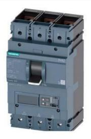
CIRCUIT BREAKER 3VA2 IEC FRAME 400 BREAKING CAPACITY CLASS C ICU=110KA @ 415 V 3-POLE, LINE PROTECTION ETU550, LSI, IN=400A OVERLOAD PROTECTION IR=160A ...400A SHORT CIRCUIT PROTECTION ISD=0,6..10X IN, II=1,5..10X IN NEUTRAL PROTECTION OPTIONAL WITH EXT. CT;UPTO 160% BUSBAR CONNECTION
