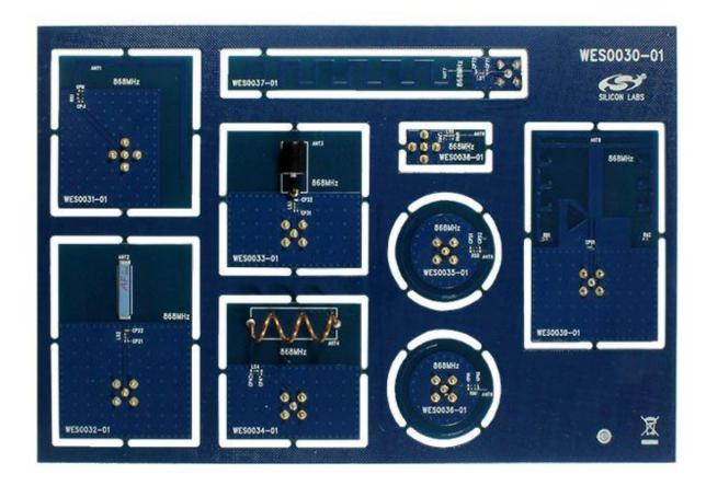
The antenna matrix is intended to simplify antenna design and selection. The antenna designs can be copied into any design after evaluation of various types of antennas in the matrix for the 868 MHz frequency band.
