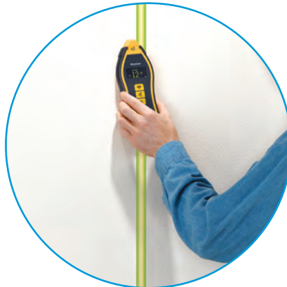
Finds Conductors in Walls, Ceilings and Floors
