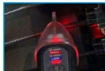
Presence of Voltage Indicated by a Flashing Red LED & Audible Tone
