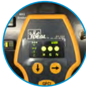
Displays H N G polarity
