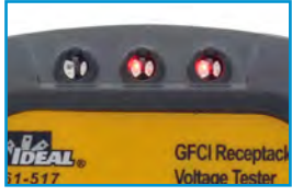
Red Lights Indicate Incorrect Wiring
