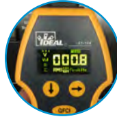
Displays neutral to ground voltage
