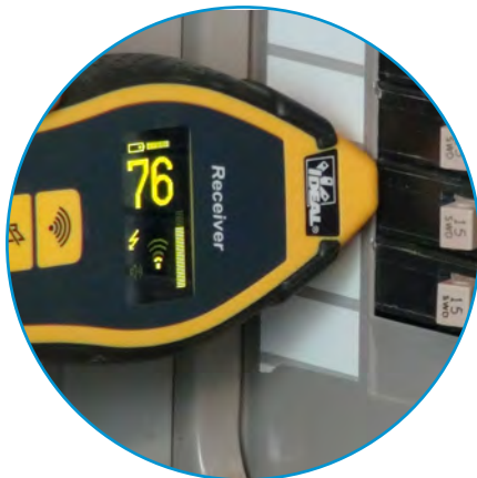
Finding Breakers or Fuses
