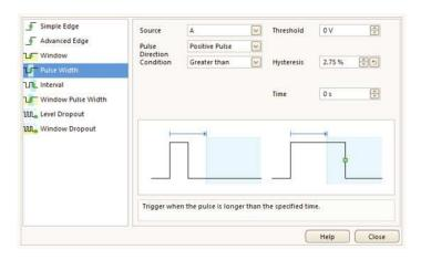
For over 20 years Pico have been pioneering the use of full digital triggering using the actual digitized data. This reduces trigger errors and allows our oscilloscopes to trigger on the smallest signals, even at the full bandwidth. All triggering is digital, resulting in high threshold resolution within programmable hysteresis and optimal waveform stability.
