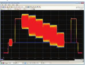
Advanced display modes allow you to see old and new data superimposed, with new data in a brighter color or shade. This makes it easy to see glitches and dropouts and to estimate their relative frequency. Choose between analog persistence, digital color, or custom display modes.
