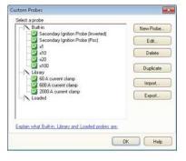
The custom probes menu allows you to correct for gain, attenuation, offsets and nonlinearities of probes and transducers, or convert your waveform data to different units such as current, scaled voltage, temperature, pressure, power or dB. Definitions can be saved to
