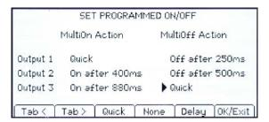
By default these turn all three outputs on or off simultaneously, but they can also be set to operate any combination of outputs in a user defined sequence with delays between 10 milliseconds and 20 seconds.
