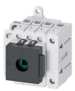
Switch disconnector 3LD3, main switch 3-polig + N, lu 25A operational switch at AC-23 A at 400 V 9,0 kW Distribution board mounting Base mounting without knob-operated mechanism with auxiliary 1NO+1NC
