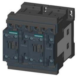
REV. COMB., AC3, 15KW/400V DC24V 3-POLE, SZ S0 SCREW TERMINAL ELECTR. AND MECH. INTERLOCK 2NO INTEGR.
