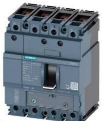
CIRCUIT BREAKER 3VA1 IEC FRAME 160 BREAKING CAPACITY CLASS H ICU=70KA @ 415 V 4-POLE, LINE PROTECTION TM240, ATAM, IN=100A OVERLOAD PROTECTION IR=70A ...100A SHORT CIRCUIT PROTECTION II=5...10 X IN NEUTRAL UNPROTECTED BUSBAR CONNECTION
