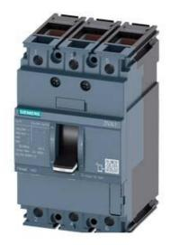
CIRCUIT BREAKER 3VA1 IEC FRAME 160 BREAKING CAPACITY CLASS S ICU=36KA @ 415 V 3-POLE, LINE PROTECTION TM210, FTFM, IN=20A OVERLOAD PROTECTION IR=20A FIXED SHORT CIRCUIT PROTECTION II=16 X IN CABLE CONNECTION
