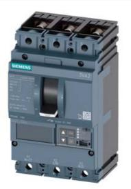
CIRCUIT BREAKER 3VA2 IEC FRAME 160 BREAKING CAPACITY CLASS C ICU=110KA @ 415 V 3POLE, LINE PROTECTION ETU860, LSIG, IN=100A OVERLOAD PROTECTION IR=40A ...100A SHORT CIRCUIT PROTECTION ISD=0,6..10X IN, II=1,5..12X IN NEUTRAL PROTECTION OPTIONAL WITH EXT. CT,UPTO 160% GROUNDFAULT, SWITCHABLE IG=0,2... 1 X IN, TG=0,050,8MS BUSBAR CONNECTION
