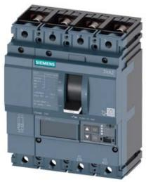
CIRCUIT BREAKER 3VA2 IEC FRAME 160 BREAKING CAPACITY CLASS L ICU=150KA @ 415 V 4POLE, LINE PROTECTION ETU850, LSI, IN=160A OVERLOAD PROTECTION IR=64A ...160A SHORT CIRCUIT PROTECTION ISD=0,6..10X IN, II=1,5..10X IN NEUTRAL PROTECTION ADJUSTABLE (OFF, UPTO 100%) BUSBAR CONNECTION
