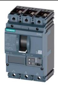
CIRCUIT BREAKER 3VA2 IEC FRAME 160 BREAKING CAPACITY CLASS C ICU=110KA @ 415 V 3POLE, LINE PROTECTION ETU560, LSIG, IN=40A OVERLOAD PROTECTION IR=16A ...40A SHORT CIRCUIT PROTECTION ISD=0,6..10X IN, II=1,5..12X IN NEUTRAL PROTECTION OPTIONAL WITH EXT. CT,UPTO 160% GROUNDFAULT, SWITCHABLE IG=0,2... 1 X IN, TG=0,050,8MS BUSBAR CONNECTION
