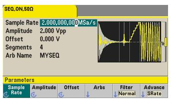
Waveform generator display of the desired sequence.
