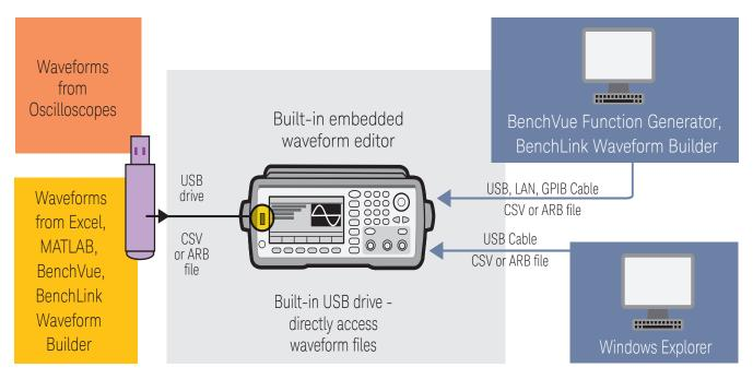
Multiple interfaces provide flexibility for creating and downloading waveforms.
