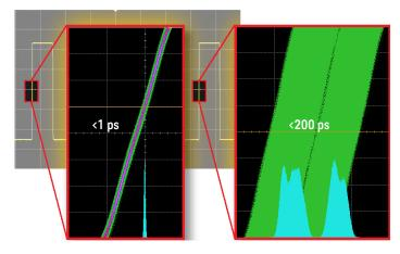
Trueform technology shown on the left significantly improves jitter performance compared to a traditional function generator shown on the right.
