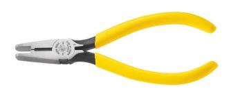
Crimps and seats Scotchlok UG, UR and UY connectors. Hot-riveted joint for smooth action and no handle wobble. Curved handles for greater control. Induction hardened side-cutting knives for long life. Spring-loaded action for self-opening. Scotchlok is a registered trademark of 3M.
