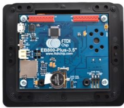
Figure 2.1 VM800P35A Module Profile 3.5" Display Version
