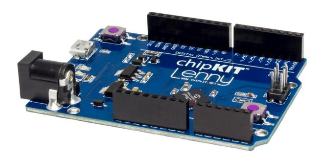
The chipKIT Lenny was inspired by the Arduino Leonardo, and adds additional capabilities afforded by its 32-bit microcontroller. The Lenny has 27 available I/O lines, 6 of which can be used as analog inputs. Based on the 32-bit PIC32MX270F256D microcontroller, operating at 3.3 volts and 40 MHz. Direct access to the USB peripheral controller enables the Lenny to emulate many types of USB devices; note that this functionality will be available in a future library.
