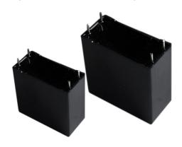
Type 953B radial leaded metallized polypropyene capacitors are designed for UPS systems and other AC output filtering applications. With an integrated fused metallization pattern, this product features UL 810 recognition for fail-safe operation at temperatures up to 85 °C.
