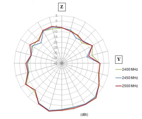
Figure 14. 2D Radiation Pattern of the WS.02 Antenna with standard 2 meter cable
