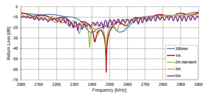
*Figure 4.* Return Loss of the Hercules WS.02 antenna with different length CFD200 cable on 30 x 30cm ground plane
