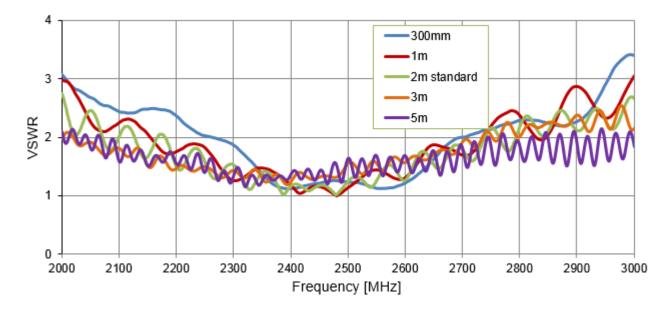
*Figure 6.* VSWR of the Hercules WS.02 antenna with different length CFD200 cable on 30 x 30cm ground plane
