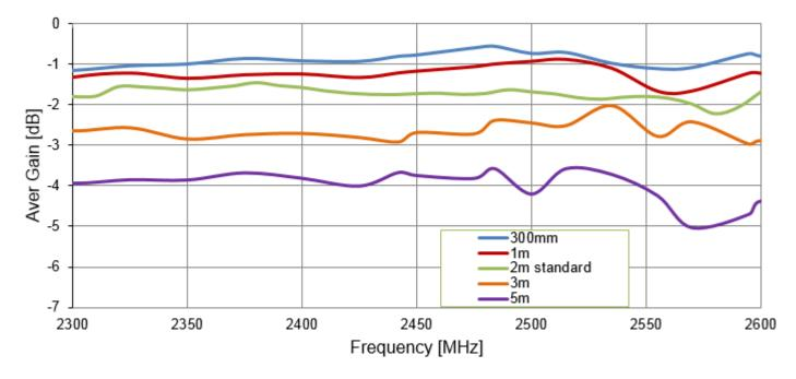
*Figure 12.* Average Gain of the Hercules WS.02 with different length CFD200 cable on 30 x 30 cm ground plane
