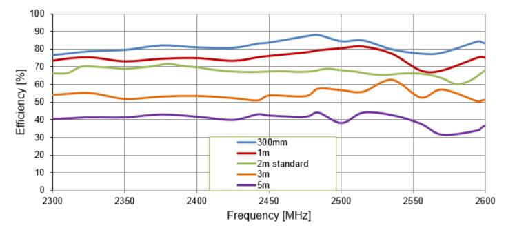
*Figure 8.* Efficiency of the Hercules WS.02 antenna with different length CFD200 cable on 30 x 30 cm ground plane
