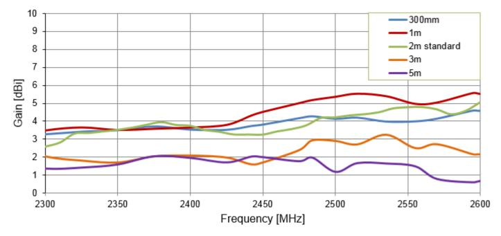
*Figure 10.* Peak Gain of the Hercules WS.02 antenna with different length CFD200 cable on 30 x 30 cm ground plane
