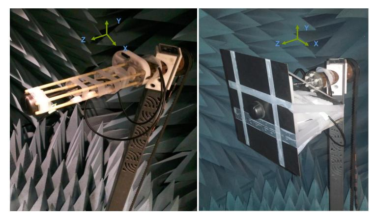
Figure 2. Peak gain, efficiency and radiation pattern measurements
