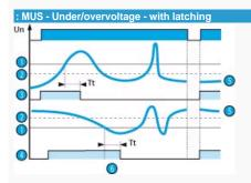
If "with memory" mode has been selected, the relay opens and stays in this position when threshold crossing is detected. The power supply must be disconnected to reset the product.
