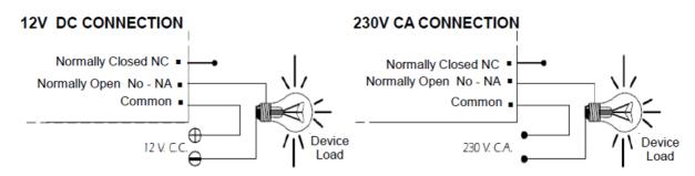
**ABOUT THE OUTPUT:** During operation of the circuit, and according to its load, it could happen fluctuation or an incorrect output performance. If this happens, install a circuit sparking between the two relay contacts used in this connection, as shown in the drawing.
