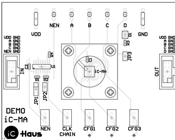
Figure 1: Component side of MA1D board
