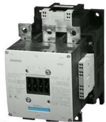
CONTACTOR, 132KW/400V/AC-3 AC(40...60HZ)/DC OPERATION UC 96-127V AUXILIARY CONTACTS 2NO+2NC 3-POLE, SIZE S10 BAR CONNECTIONS ELECTRONIC OPERATING MECHANISM WITH 24 V DC PLC INTERFACE CAGE CLAMP TERMINAL
