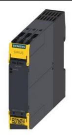
SIRIUS SAFETY RELAY OUTPUT EXTENSION 4RO WITH RELAY ENABLING CIRCUITS 4 NO CONTACTS + RELAY FEEDBACK CIRCUIT 1 NC CONTACT US = 24 V AC SCREW CONNECTION
