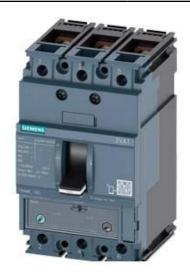
CIRCUIT BREAKER 3VA1 IEC FRAME 160 BREAKING CAPACITY CLASS S ICU=36KA @ 415 V 3-POLE, LINE PROTECTION TM240, ATAM, IN=125A OVERLOAD PROTECTION IR=87,5A ...125A SHORT CIRCUIT PROTECTION II=5...10 X IN BUSBAR CONNECTION
