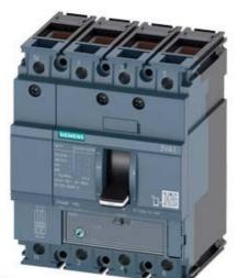
CIRCUIT BREAKER 3VA1 IEC FRAME 160 BREAKING CAPACITY CLASS M ICU=55KA @ 415 V 4-POLE, LINE PROTECTION TM220, ATFM, IN=160A OVERLOAD PROTECTION IR=112A ...160A SHORT CIRCUIT PROTECTION II=10 X IN NEUTRAL PROTECTION 100% CABLE CONNECTION
