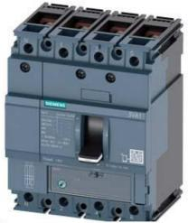
CIRCUIT BREAKER 3VA1 IEC FRAME 160 BREAKING CAPACITY CLASS H ICU=70KA @ 415 V 4-POLE, LINE PROTECTION TM220, ATFM, IN=160A OVERLOAD PROTECTION IR=112A ...160A SHORT CIRCUIT PROTECTION II=10 X IN NEUTRAL UNPROTECTED BUSBAR CONNECTION
