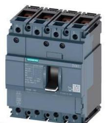
CIRCUIT BREAKER 3VA1 IEC FRAME 160 BREAKING CAPACITY CLASS N ICU=25KA @ 415 V 4-POLE, LINE PROTECTION TM210, FTFM, IN=80A OVERLOAD PROTECTION IR=80A FIXED SHORT CIRCUIT PROTECTION II=10 X IN NEUTRAL UNPROTECTED BUSBAR CONNECTION
